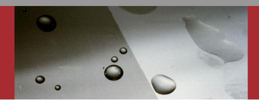
1 Stainless steel surface, with hybrid polymer ORMOCER® coating on the left-hand side: water beads simply roll off and fingerprints are barely visible in contrast to the uncoated right-hand side.
