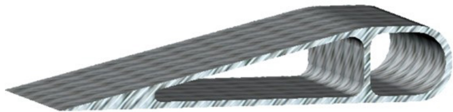
© Rolls-Royce Deutschland Ltd & Co KG Airfoil geometry to be translated into a textile ceramic fiber preform.
