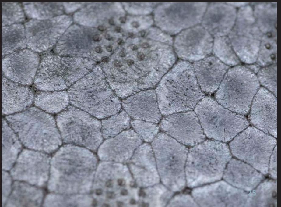
Uniform pore structure of an inductively foamed polystyrene
